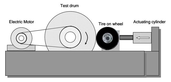
Figure 4. Typical Test Configuration for Rolling Resistance Measurements
