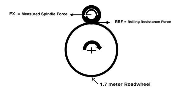
Figure 5. Force Method Rolling Resistance
